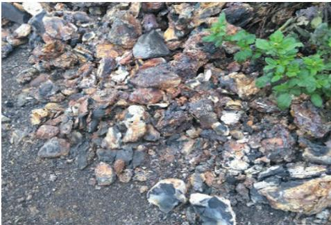
*Coal does not combust completely*
