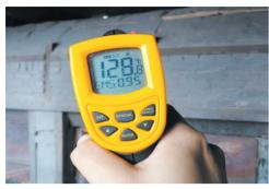
Insulation of Tea Withering machine does not function well.
