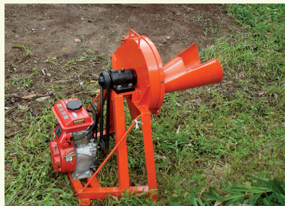
Petrol powered rattan leaf cutting machine
