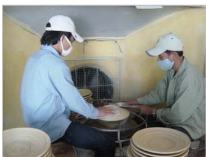
Dust extractors were installed in the Jute Company, Nam Dinh
