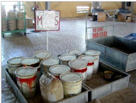
Application of cleaner production does not need to be complicated. Providing a tray for chemicals can be an option
